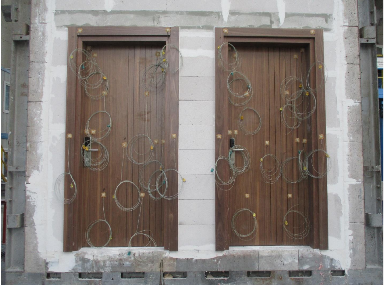
Photo C1: Unexposed side for the test specimens before the test.
