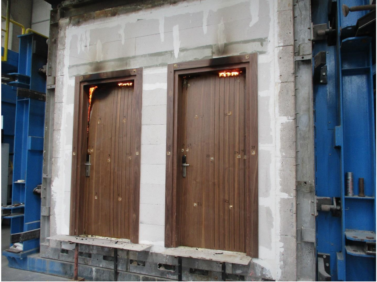
Photo C3: Unexposed side for the test specimens after the test.
