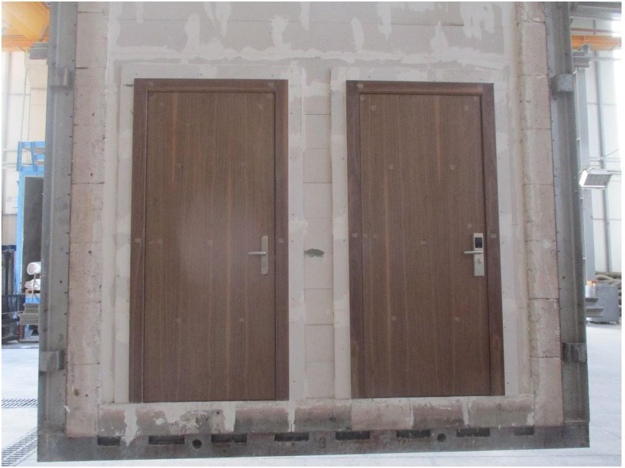
Photo C2: Exposed side for the test specimens before the test.
